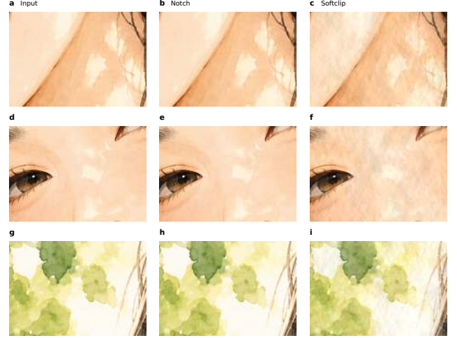
Figure 4. Input windows, selective notch outputs and radial soft-clipping outputs for matched skin, eyes and foliage regions.
